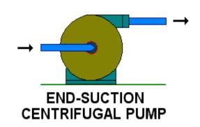
Almost all portable pumps are end-suction centrifugals. If the pump isn't one of the next two types, then chances are it is an end-suction centrifugal. This type of pump needs to be installed on a pad above the high water level if pumping from a lake or river.
