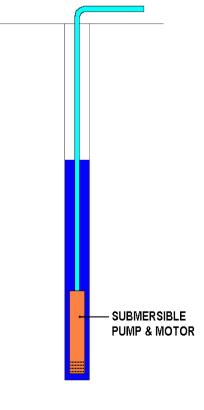
Because the power cord runs down to the pump through the water it is very important that it be protected from accidental damage
